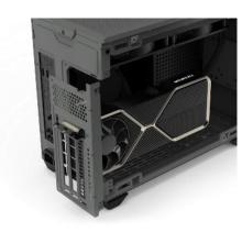
**Quick Install GPU Panel**The exclusive removable GPU
